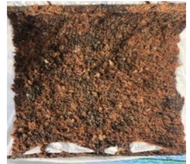
Untreated sample after 91 days in sea
