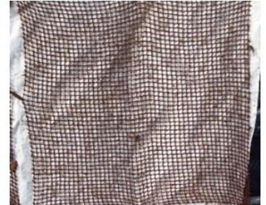
Untreated sample after 91 days in sea
